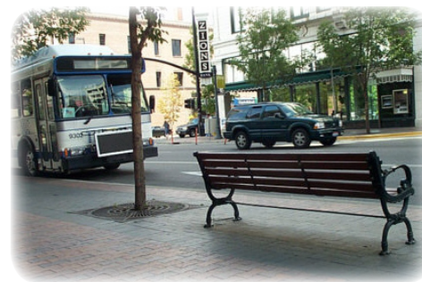
Example of a bench-only stop in Boise, Idaho. The bench is not located on the bus landing pad and does not impede access to the stop.
