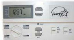
Do this automatically without sacrificing comfort by installing an automatic setback or programmable thermostat. Adjust the times you turn on the heating or air-conditioning according to a pre-set schedule. As a result, the equipment doesn't operate as much when you are asleep or when the house, or a part of it, is not occupied.
